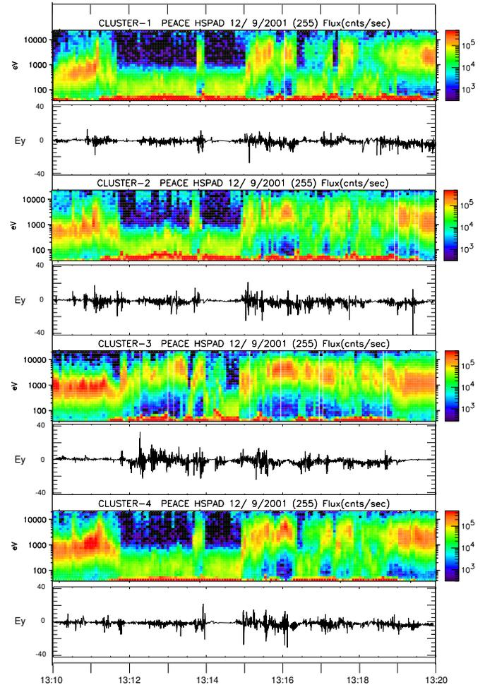
**Fig. 4.** Figure 5 shows the electron flux, integrated over pitch angle, together with the electric field  $E_y$ . Largest  $E_y$  fluctuations generally correspond to bursts of energetic electrons.
