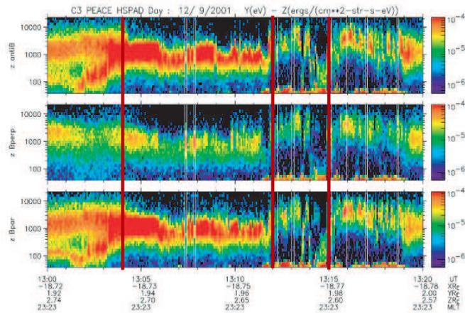
**Fig. 3.** s/c3 PEACE Electron energy fluxes in 3 directions: opposite (top), perpendicular (middle), and parallel (bottom) to  $B$ .
