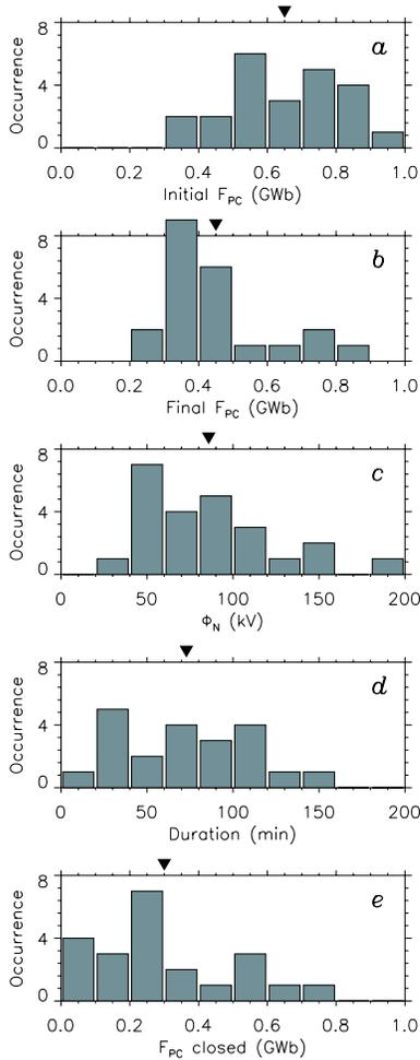
**Fig. 2.** The characteristics of 25 nightside reconnection bursts identified during 73 hours of observations. (a) The open flux  $F_{PC}$  at onset of each event; (b)  $F_{PC}$  at the end of each event; (c) the reconnection rate and (d) duration of each event; (e) the amount of flux closed during each event. Arrows indicate the average of each distribution.
